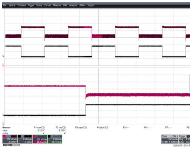
Figure 38 – Transient Response. 265 VAC, 9.0 V, 0 - 3 A Load Step. V_{MIN} : 9.159V, V_{MAX} : 8.708 V. Upper: V_{OUT} , 0.2 V / div., 200 ms / div. Lower: I_{LOAD} , 2 A / div. Zoom: 20 ms / div.
