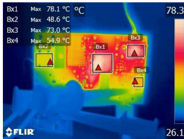
Figure 110 – Bottom Components, Ambient = 26.3 °C. Bx1: InnoSwitch3, U1 = 78.1 °C. Bx2: Bridge Rectifier, BR1 = 48.6 °C. Bx3: SR FET, Q2 = 73 °C. Bx4: Bus Switch, Q3 = 54.9 °C.
