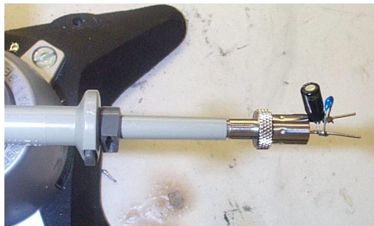
Figure 80 – Oscilloscope Probe with Probe Master ( www.probemaster.com ) 4987A BNC Adapter. (Modified with wires for ripple measurement, and two parallel decoupling capacitors added)
