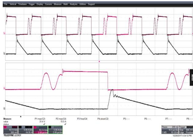
Figure 76 – SR FET Drain Voltage and Current Waveforms. 115 VAC, 11.0 V, 3 A Load, (31.4 V MAX ). Upper: V SR_DRAIN , 10 V, 10 μs / div. Lower: I SR_DRAIN , 5 A / div. Zoom: 2 μs / div.
