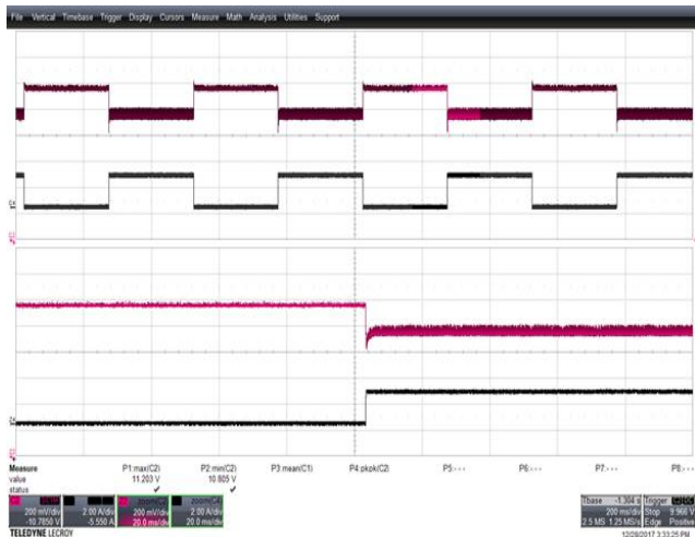
Figure 45 – Transient Response. 230 VAC, 11.0 V, 0 – 2.45 A Load Step. V_{MIN} : 10.805 V, V_{MAX} : 11.203 V. Upper: V_{OUT} , 0.2 V / div., 200 ms / div. Lower: I_{LOAD} , 2 A / div. Zoom: 20 ms / div.
