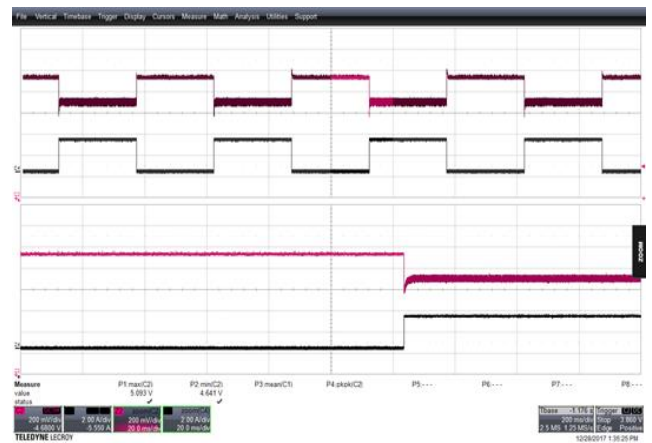
Figure 34 – Transient Response. 265 VAC, 5.0 V, 0 - 3 A Load Step. V MIN : 4.641 V, V MAX : 5.093 V. Upper: V OUT , 0.2 V / div., 200 ms / div. Lower: I LOAD , 2 A / div. Zoom: 20 ms / div.
