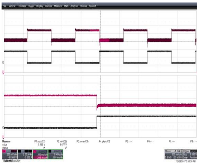
Figure 37 – Transient Response. 230 VAC, 9.0 V, 0 - 3 A Load Step. V_{MIN} : 8.677 V, V_{MAX} : 9.169 V. Upper: V_{OUT} , 0.2 V / div., 200 ms / div. Lower: I_{LOAD} , 2 A / div. Zoom: 20 ms / div.
