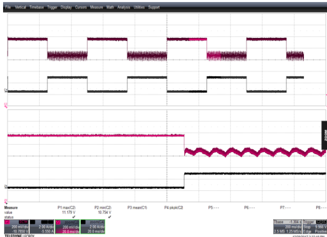
Figure 43 – Transient Response. 85 VAC, 11.0 V, 0 – 2.45 A Load Step. V_{MIN} : 10.754 V, V_{MAX} : 11.179 V. Upper: V_{OUT} , 0.2 V / div., 200 ms / div. Lower: I_{LOAD} , 2 A / div. Zoom: 20 ms / div.
