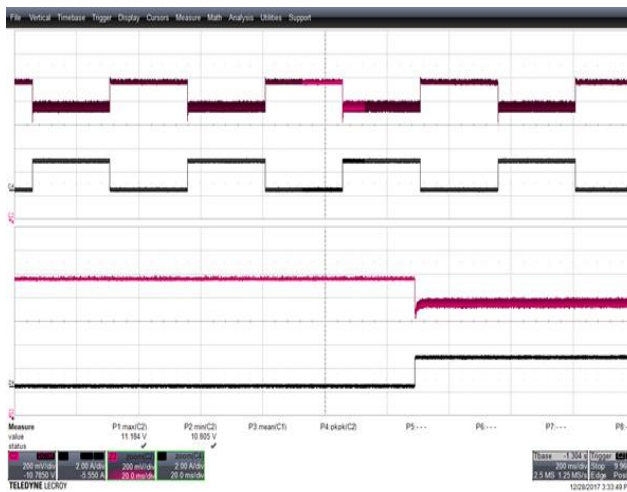
Figure 46 – Transient Response. 265 VAC, 11.0 V, 0 – 2.45 A Load Step. V_{MIN} : 10.805 V, V_{MAX} : 11.184 V. Upper: V_{OUT} , 0.2 V / div., 200 ms / div. Lower: I_{LOAD} , 2 A / div. Zoom: 20 ms / div.
