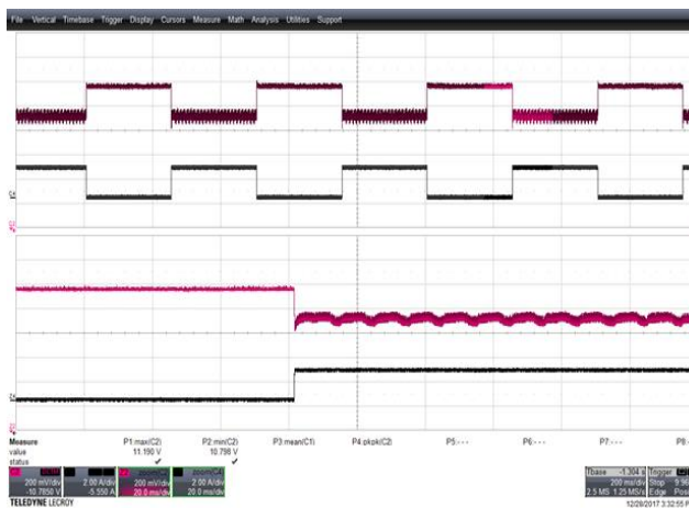
Figure 44 – Transient Response. 115 VAC, 11.0 V, 0 – 2.45 A Load Step. V_{MIN} : 10.798 V, V_{MAX} : 11.190 V. Upper: V_{OUT} , 0.2 V / div., 200 ms / div. Lower: I_{LOAD} , 2 A / div. Zoom: 20 ms / div.
