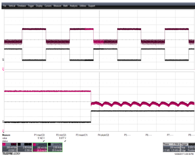
Figure 35 – Transient Response. 85 VAC, 9.0 V, 0 - 3 A Load Step. V_{MIN} : 8.677 V, V_{MAX} : 9.142 V. Upper: V_{OUT} , 0.2 V / div., 200 ms / div. Lower: I_{LOAD} , 2 A / div. Zoom: 20 ms / div.
