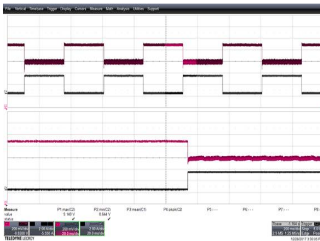
Figure 36 – Transient Response. 115 VAC, 9.0 V, 0 - 3 A Load Step. V_{MIN} 8.644 V, V_{MAX} : 9.149 V. Upper: V_{OUT} , 0.2 V / div., 200 ms / div. Lower: I_{LOAD} , 2 A / div. Zoom: 20 ms / div.
