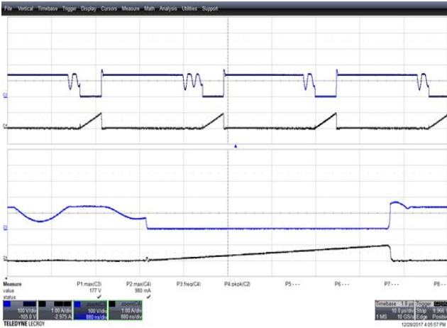
Figure 55 – Drain Voltage and Current Waveforms. 85 VAC, 3.0 V, 3 A Load, (177 V_{MAX} ). Upper: V_{DRAIN} , 100 V, 10 \mu s / div. Lower: I_{DRAIN} , 1 A / div. Zoom: 880 ns / div.
