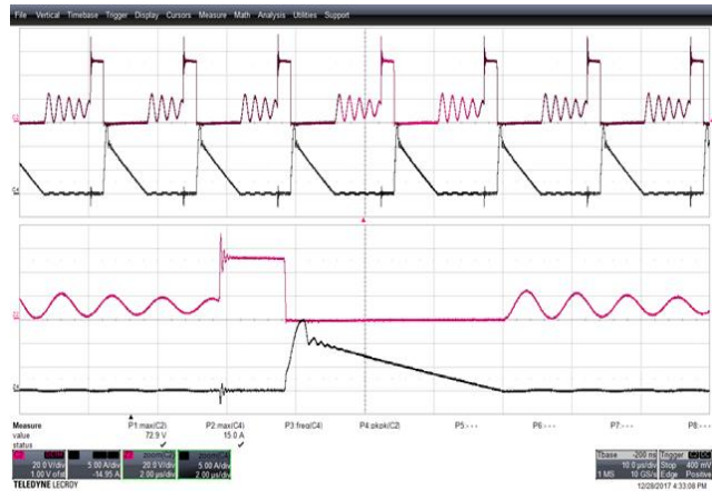
Figure 78 – SR FET Drain Voltage and Current Waveforms. 265 VAC, 11.0 V, 3 A Load, (72.9 V MAX ). Upper: V SR_DRAIN , 20 V, 10 μs / div. Lower: I SR_DRAIN , 5 A / div. Zoom: 2 μs / div.
