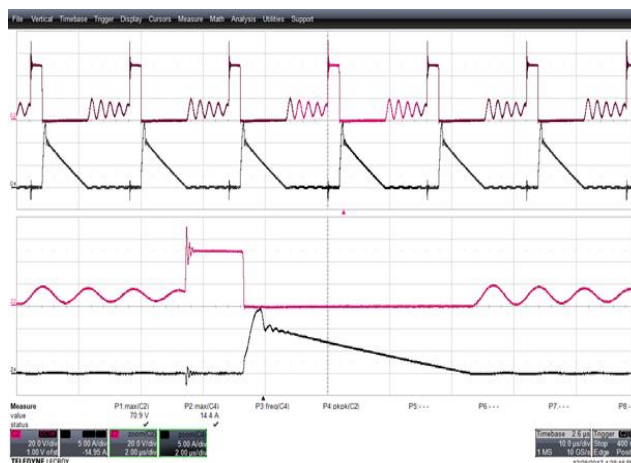
Figure 70 – SR FET Drain Voltage and Current Waveforms. 265 VAC, 9.0 V, 3 A Load, (70.9 V MAX ). Upper: V SR_DRAIN , 20 V, 10 μs / div. Lower: I SR_DRAIN , 5 A / div. Zoom: 2 μs / div.
