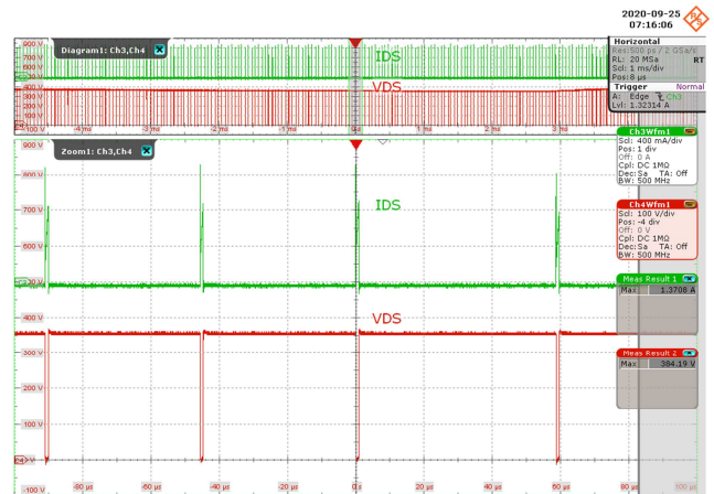
Figure 20 – Drain Voltage and Current Waveforms. 115 VAC, 550 mA Output. Upper: I_{DS} , 400 mA / div. Lower: V_{DS} , 40 V / div., 20 \mu s / div. I_{DS(MAX)} = 1.17 A, V_{DS(MAX)} = 174.2 V.
