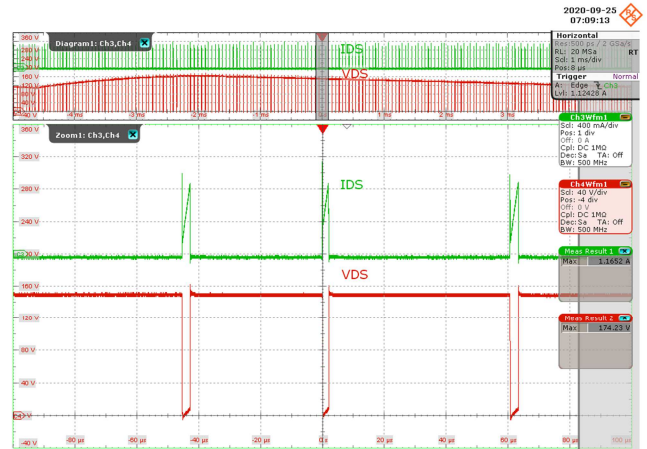
Figure 20 – Drain Voltage and Current Waveforms. 115 VAC, 550 mA Output. Upper: I_{DS} , 400 mA / div. Lower: V_{DS} , 40 V / div., 20 \mu s / div. I_{DS(MAX)} = 1.17 A, V_{DS(MAX)} = 174.2 V.
