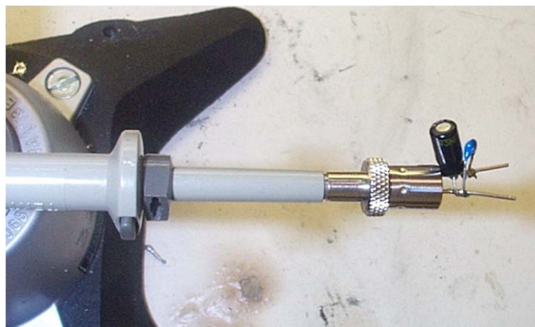
Figure 43 – Oscilloscope Probe with Probe Master ( www.probemaster.com ) 4987A BNC Adapter. (Modified with Wires for Ripple Measurement, and Two Parallel Decoupling Capacitors added)
