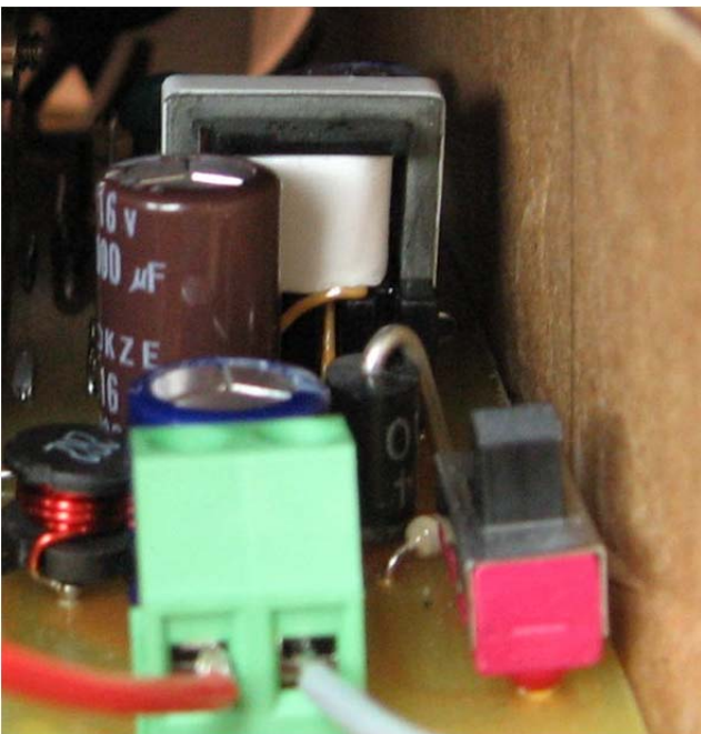
Figure 56 – Standby Output Rectifier D16, Visible Light View.
