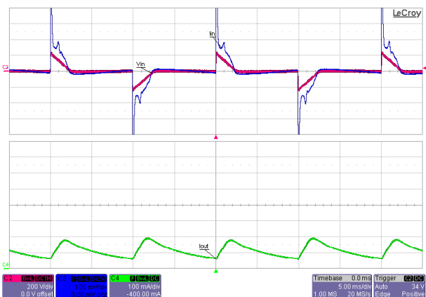
Figure 82 – 240 VAC / 50 Hz, (Germany) Ove Dimmer at Minimum TRIAC Conduction. Load:36 V LED String. Ch2:V IN , 200 V / div. Ch3:I IN , 100 mA / div. Ch4:I OUT , 100 mA / div. Time Scale:5 ms / div.
