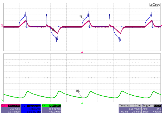
Figure 84 – 240 VAC / 50 Hz, (Germany) Busch 691 U-101 Dimmer at Minimum TRIAC Conduction. Load:36 V LED String. Ch2:V IN , 200 V / div. Ch3:I IN , 100 mA / div. Ch4:I OUT , 100 mA / div. Time Scale:5 ms / div.
