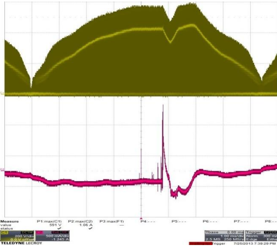
Figure 91 –265 VAC / 60 Hz, 36 V Load, V_{DS} = 591 V_{PK} (+) 500 V Diff. Line Surge at 90°. Ch1: V_{DS} , 200 V / div. Ch2: I_{IN} , 500 mA / div. Time Scale: 1 \mu s / div.
