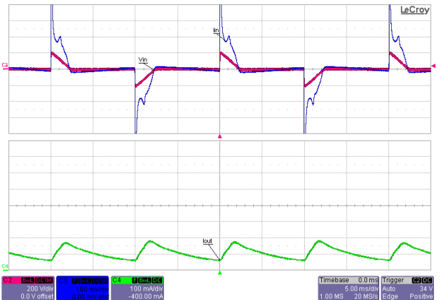
Figure 72 – 240 VAC / 50 Hz, (Germany) Busch 2250 600 W Dimmer at Minimum TRIAC Conduction. Load:36 V LED String. Ch2:V IN , 200 V / div. Ch3:I IN , 100 mA / div. Ch4:I OUT , 100 mA / div. Time Scale:5 ms / div.
