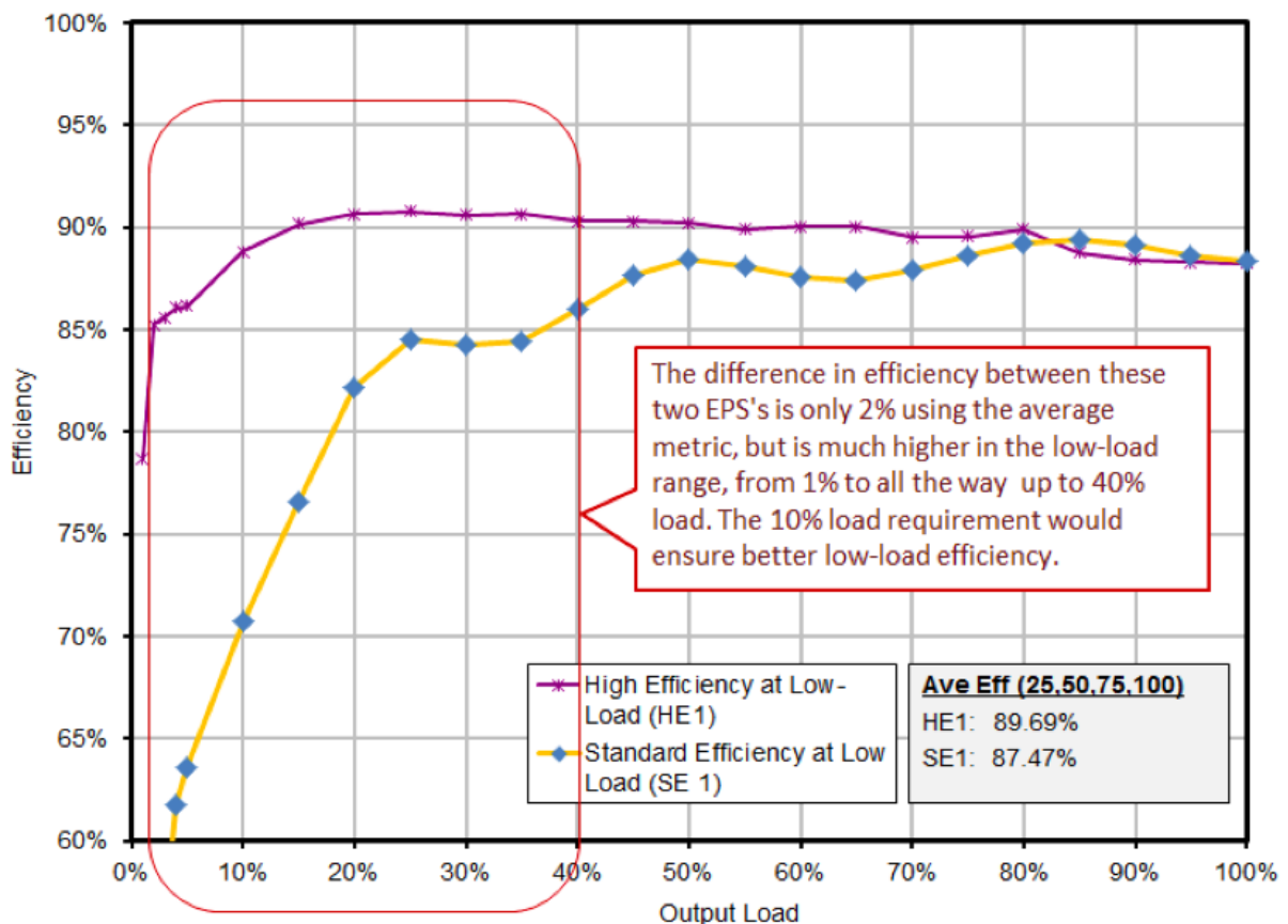
Figure 2 – Low load efficiency variation for two EPS at 230V. 13
